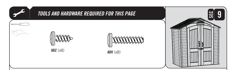
Secure the Roof Panels to the Truss and Wall Panels using four (4) 1/4" x 5/8" Pan-Head Screws (ADZ) and four (4) 1/4" x 1 1/8" Pan-Head Screws (ADZ). Repeat steps 9.3 - 9.4 for the other front Roof Panel.
