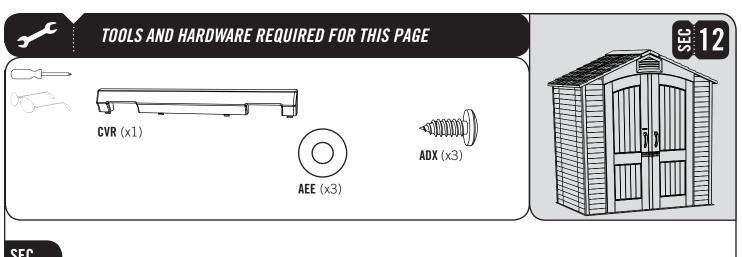
Slide the **Small Right Door Latch Cover (CVR)** down over the Right Door Latch Brackets as shown. Secure the Small Right Door Latch Cover to the Door using three (3) **#10 x 1/2" Pan-Head Screws (ADX)** and three (3) **#10 Flat Washers (AEE)**.
