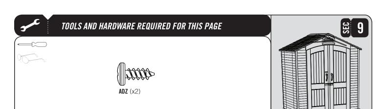
Secure the End Roof Cap to the Entry Gable using two (2) 1/4" x 5/8" Pan-Head Screws (ADZ).
