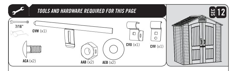
Slip the **Door Latch (CVW)** into the loops of the **Large Right Door Latch Bracket (CVU)** and the **Small Right Door Latch Bracket (CVV)** as shown.
