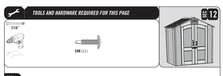
Close the Doors, and adjust the Left Door Latch Bracket up or down so the Door Latch closes easily. Once the Left Door Latch Bracket is in place, insert one (1) #10 x 3/4" Self-Drilling/Self Tapping Screw (CHK) through the small hole in the Left Door Latch Bracket, through the Left Door, and into the Square Tube inside the Door. Do not overtighten. Finally, open the Doors and tighten the Centerlock Nut (AAB) on the back of the Left Door. Finally,
