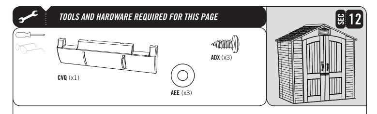
Insert the Large Right Door Latch Cover (CVQ) at an angle over the Right Door Latch Brackets as shown. Then, rotate the Cover so it's flat against the Door as shown. Secure the Large Right Door Latch Cover to the Door using three (3) #10 x 1/2" Pan-Head Screws (ADX) and three (3) #10 Flat Washers (AEE).
