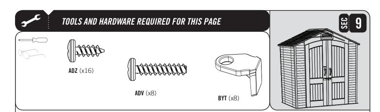
Attach the last two Roof Panels to the Shed. Secure the Rear Gable Assembly and Roof Panels together using eight (8) Gable-to-Roof Clips (BYT) (In the direction illustrated), sixteen (16) 1/4" x 5/8" Pan-Head Screws (ADZ), and eight (8) 1/4" x 1 1/8" Pan-Head Screws (ADV). The Screws (ADV) connect the tops of the Wall Panels to the bottom of the Roof Panels.
