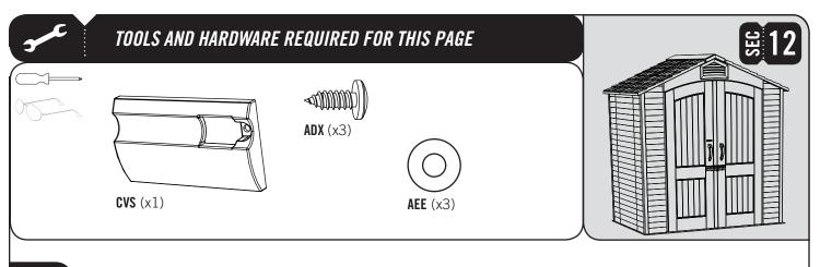
Place the **Left Door Latch Cover (CVS)** over the Left Door Latch Bracket as shown. Secure the Left Door Latch Cover to the Door using three (3) **#10 x 1/2" Pan-Head Screws (ADX)** and three (3) **#10 Flat Washers (AEE)**.
